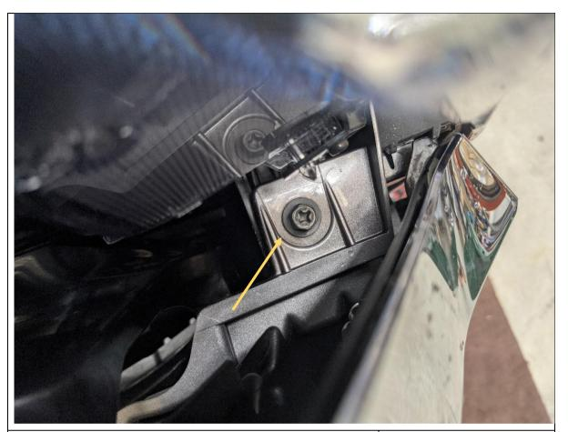
12. Remove the 2x 10mm Head/Phillips screws securing the bumper to crossmember.
