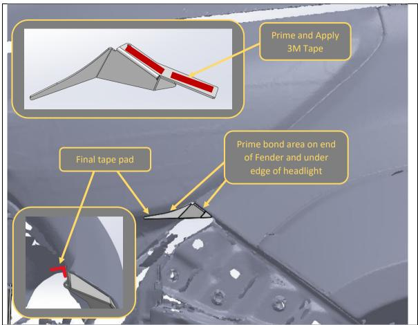
76. Using 3M primer stick from parking sensors, apply primer to end of fender panel and small headlight infill in the bonding area as shown.
