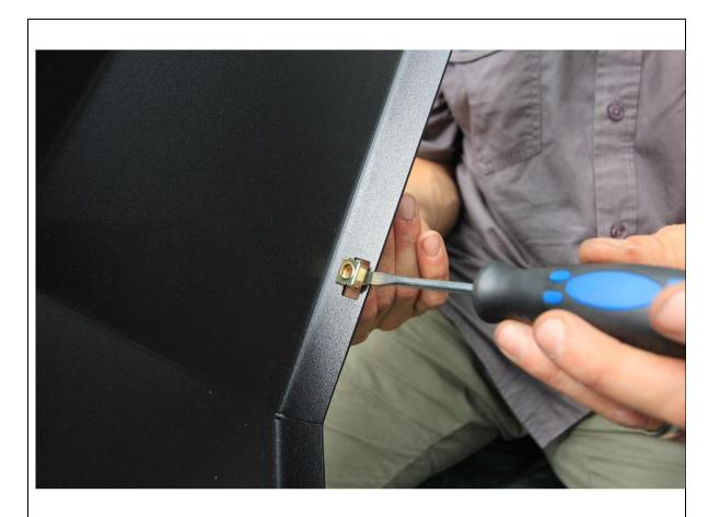
84. Insert cage nuts to square slots in bottom of wings. Seat cage nut against one edge of slot then push other edge in with flat bladed screwdriver.
