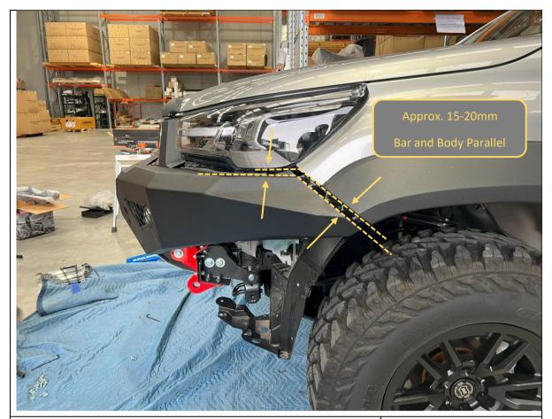
89. Align the bar with the body. Aim for 15-20mm clearance between the wing and body.
