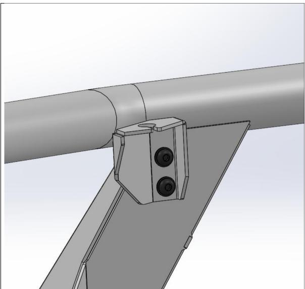
121. **Toro only.** Fit antenna brackets to Toro uprights using M8x20 black button head bolts and black washers.
