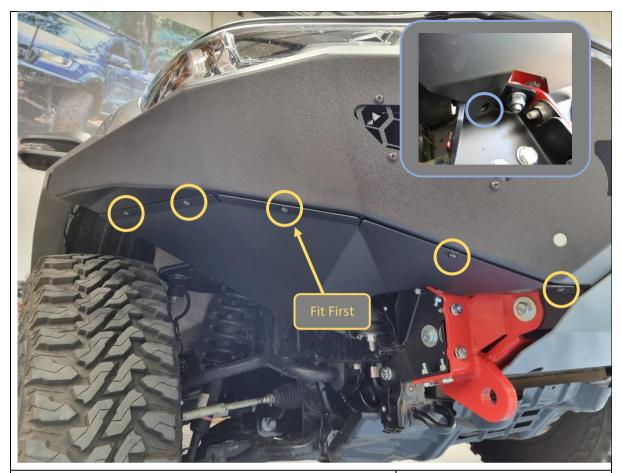
114. Fit side under panels to bar and secure with 5xM6x16 Button head bolts and M6 Flat washers, intoM6 cage nuts fitted earlier.
