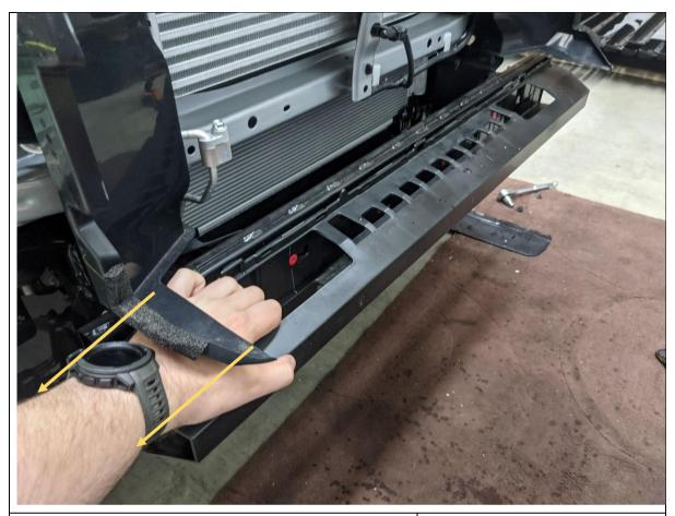
25. Remove the plastic cover from the impact beam by strongly pulling in the direction shown to release it from the clips
