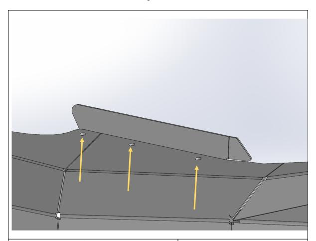
85. Fit the plastic infill panels to the bar, using supplied M6x16 Black Button head bolts, Black washers, and flange nuts.
